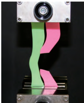
Fig. 7: addition mini Junior (intact) and Xsoft Shore A 25 (torn) exposed to equal force and tensile load
