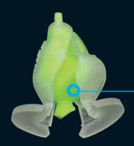
Due to the predetermined tear line and the flexible material properties, the earmould can be demolded without tools. This prevents formation of sharp-edged fragments that could damage the silicone earmould. The nominal tear line can be easily created directly in the design software (3shape, Cyfex).
