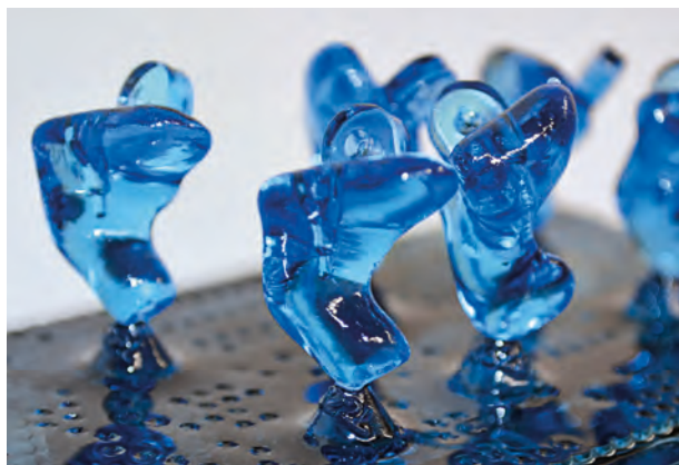
Fig. 3: Application example: Coloured plastic luxaprint® 3D mould
