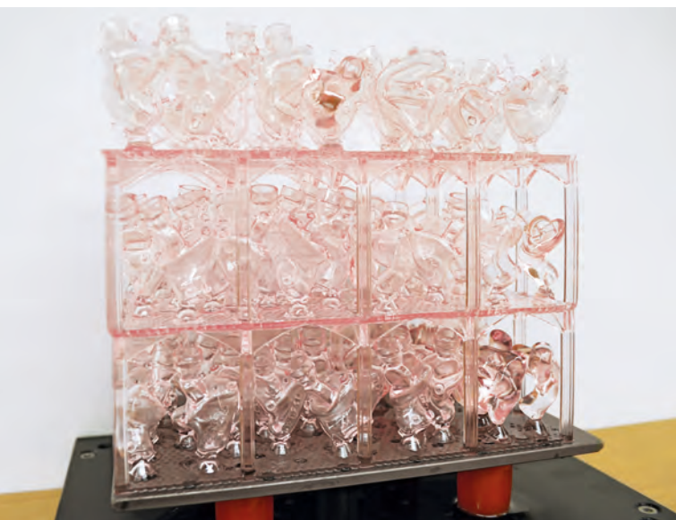
Fig. 2: Multilayer print on the HA 90
